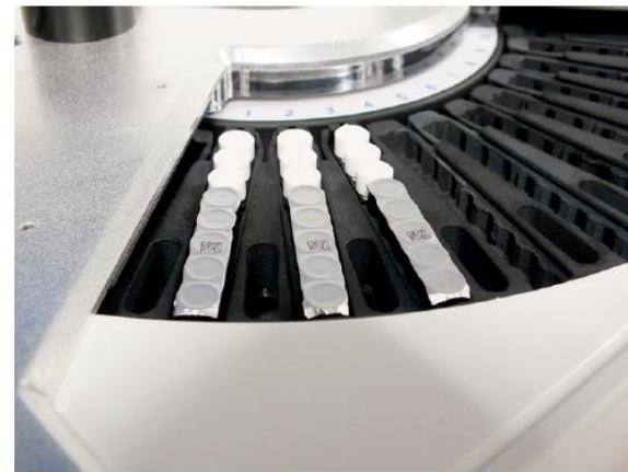
Internal barcode Monotests identified with 2D or QR barcode
