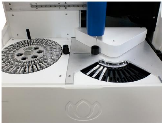
2 accessible rotors: samples and monotests
